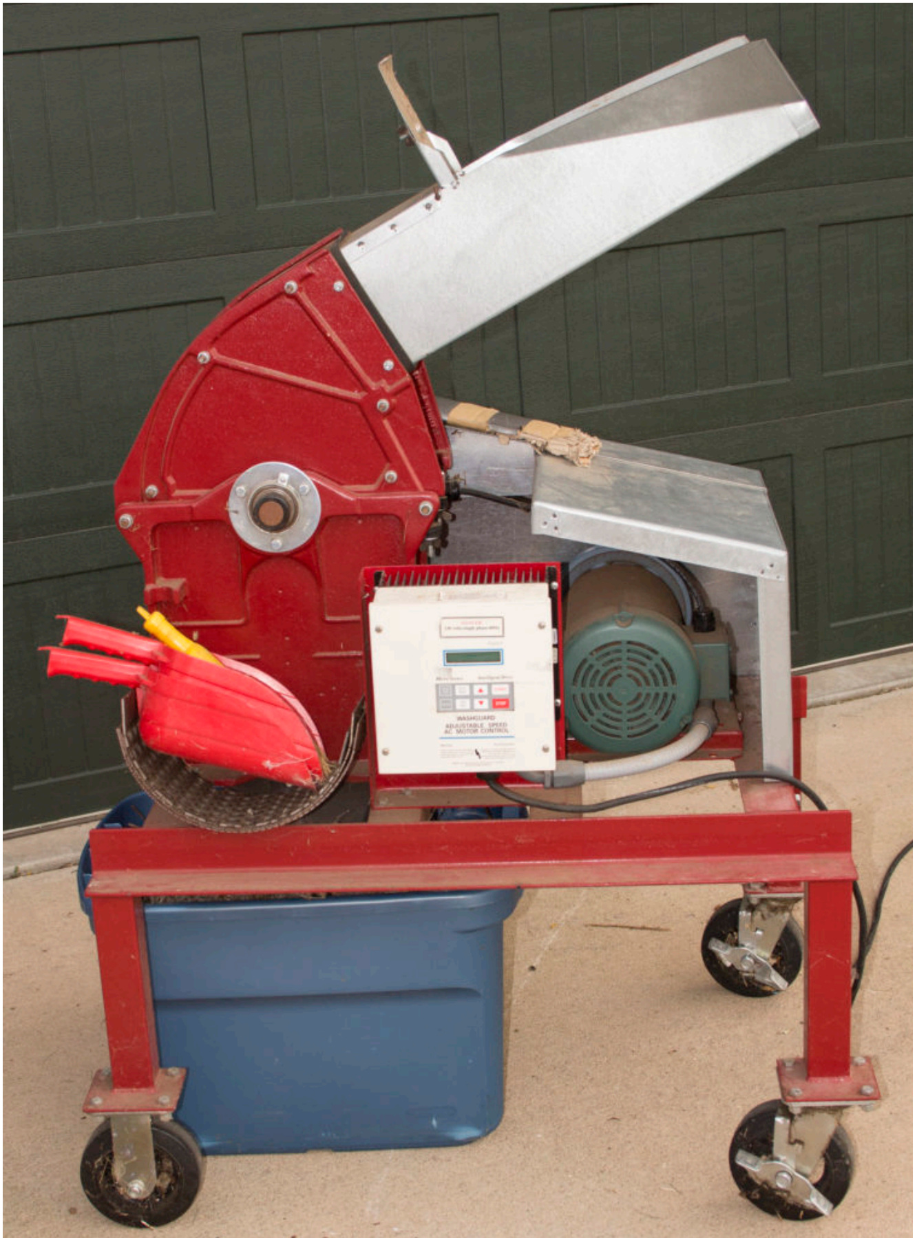
The hammermill is a work horse at our place. It's made of cast iron!
